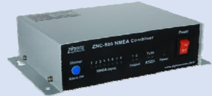
ZNC-580 has filtering function of NMEA data. The function is available to receive the specific NMEA data came from specific port, and output these data via specific port. Also it can filter out the unwanted NMEA data and reduce the traffic of combined NMEA data.
